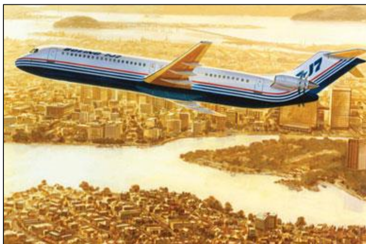
Figure 1: Boeing 7J7, a proposed design by Boeing with prop-fans as the powerhouse. (2)
